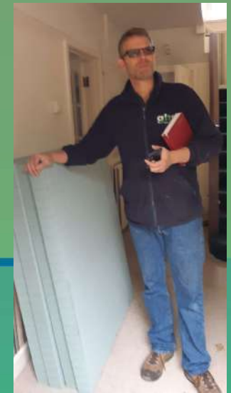
Structural insulation - Partel Alma Vert – from recycled bottles
