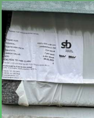
SB exp polystyrene EPS 0.031 W/mK
