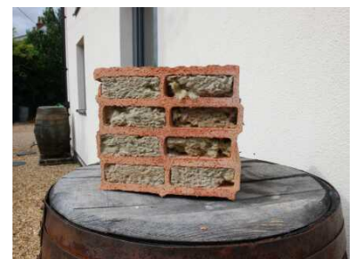
Rockwool-filled extruded clay blocks
